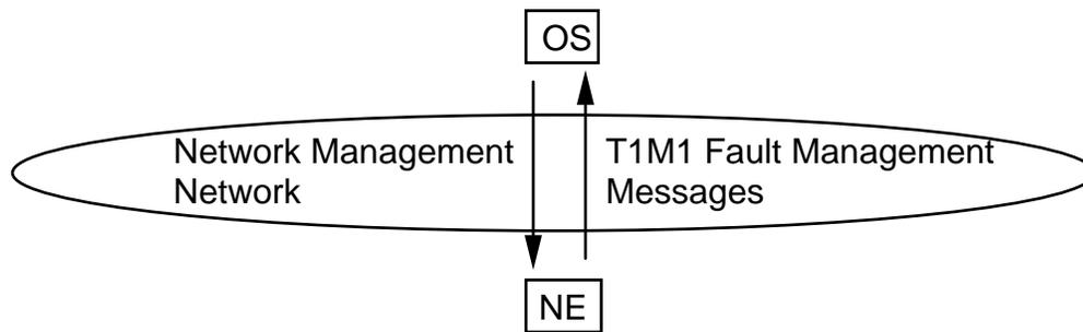
**Figure 2: Fault management functions**
